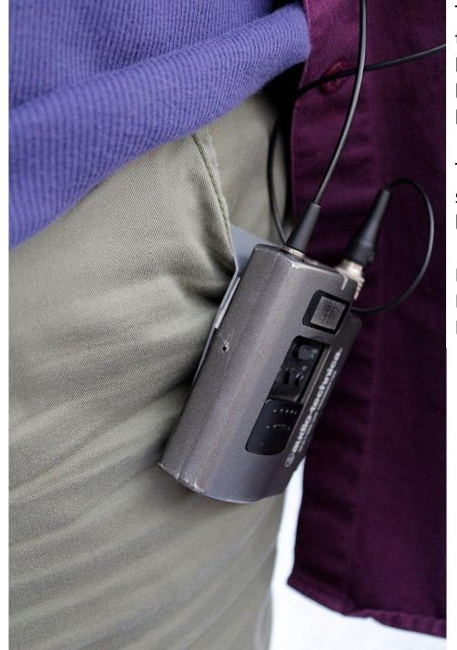
The wireless microphone transmitters use AA batteries and can be hooked over a pocket or belt.
